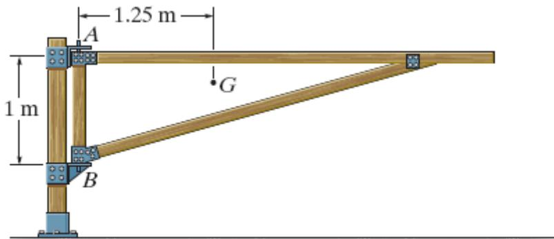
3- The overhanging beam is supported by a pin at  $A$  and the two-force strut  $BC$ . Determine the horizontal and vertical components of reaction at  $A$  and the reaction at  $B$  on the beam. ( $F_{BC} = 3916.67 \text{ N}$ ,  $A_x = 3133.33 \text{ N}$ ,  $A_y = 950 \text{ N}$ )
