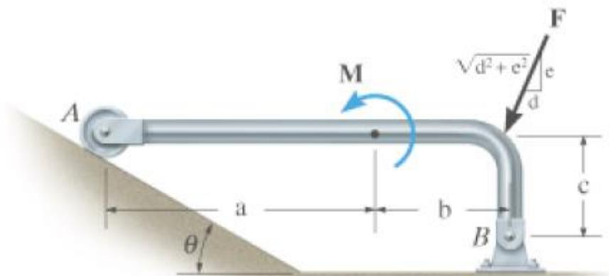
5- Determine the reactions on the bent rod which is supported by a smooth surface at  $B$  and by a collar at  $A$ , which is fixed to the rod and is free to slide over the fixed inclined rod. ( $F = 100\text{N}$ ,  $M = 20\text{N}\cdot\text{m}$ ,  $a = 0.3\text{m}$ ,  $b = 0.3\text{m}$ ,  $c = 0.2\text{m}$ ,  $d = 3$ ,  $e = 4$ ,  $f = 12$ ,  $g = 5$ )
